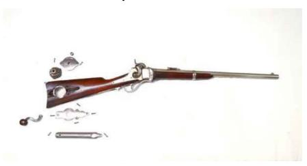
This .52-calibre Sharps New Model 1863 Carbine from the Buffalo Bill Center of the West shows an exploded view of buttstock's coffee grinder. *Buffalo Bill Center of the West*
